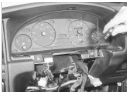
9.21 Unscrew the lower instrument panel securing screws
