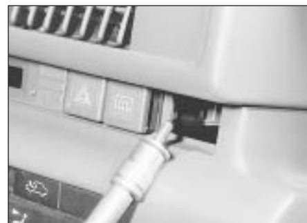
9.3a . . . and remove the visor securing screws
