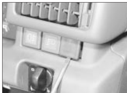
9.2 Prise out the blanking plates . . .
