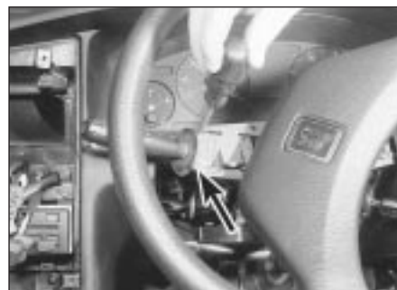
4.6a Remove the securing screws . . .
