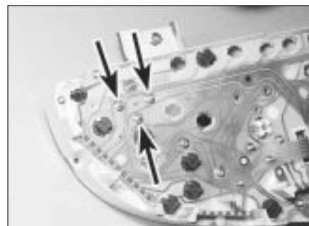
10.9 Fuel gauge securing nuts (arrowed)
