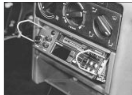
20.3 . . . then insert the removal tools . . .
