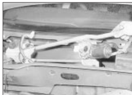
17.8c Withdrawing the windscreen wiper motor and linkage assembly
