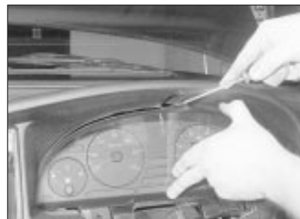
9.22 Lever the upper securing clip down . . .
