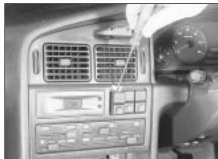
4.14 Prising out a facia-mounted switch - models from 1993
