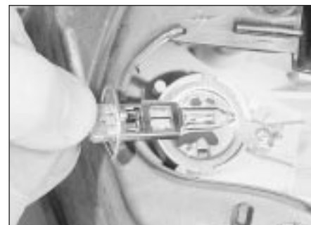
5.23b Removing a headlight-mounted driving light bulb
